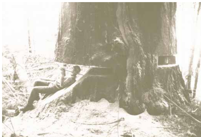
Faller checking the intended lay of the tree with a gunning stick, prior to putting in the backcut. Hydraulic jacks already set in back, ready to tip the tree over once the backcut is completed.
