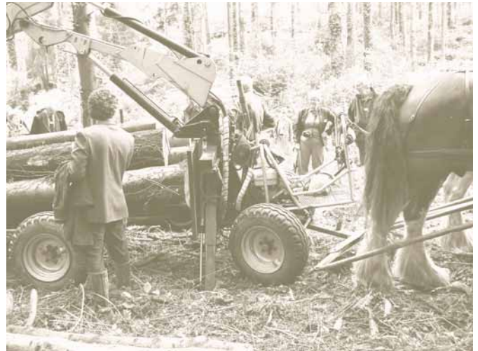
Hydraulic gear and modern logging arches enable a traditional craft to move with the times.
