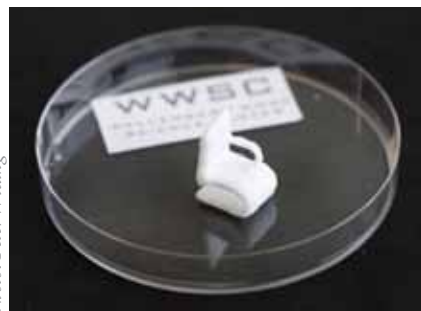
The tiny chair made of cellulose is a demonstrational object printed using the 3-D bioprinter at Chalmers University of Technology
