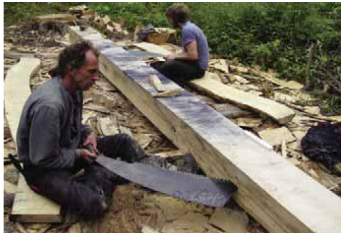
Axel and Jack sawing in tandem with Japanese Maebiki Oga saws.
