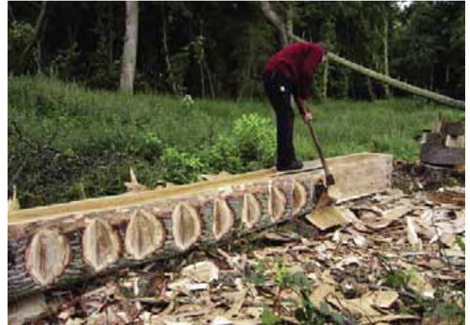
Axel rough hewing with a Breton long-handled axe.
