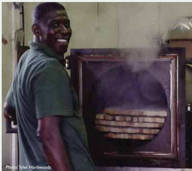
Lionel Howell, Steam Bending Operator, loading bending staves into steaming vessel.
