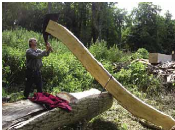
Axel saws two collars from one tree with a Maebiki Oga saw.
