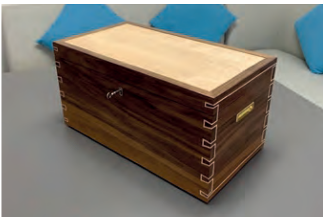
Level 3 City and Guilds Furniture Making – Tool box in Walnut and sycamore with hand cut dovetail joints
