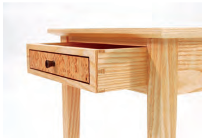
Level 2 City and Guilds Furniture Making – Small table with hand cut dovetail joints and veneer/inlay detail
