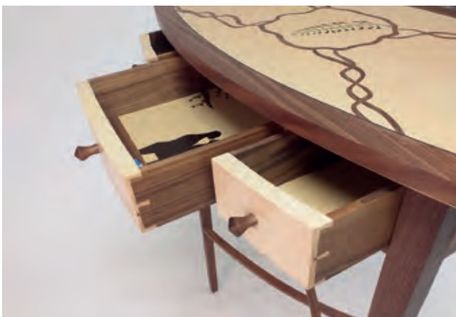
Level 3 City and Guilds Furniture Making - Side table in Walnut and Sycamore with hand cut dovetail joints
