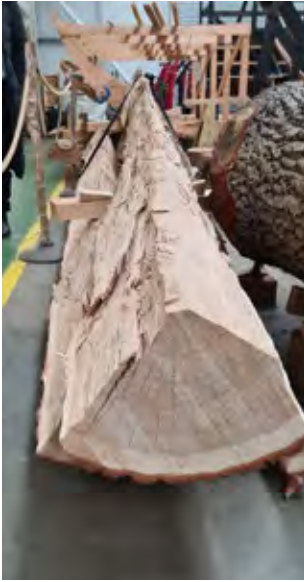
A quartered oak log cleaved by hand for planks (left); willow tree nail with Oak wedge (right)
