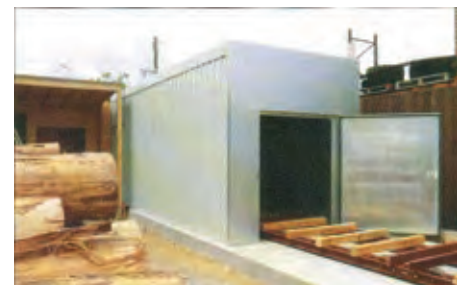
Small timber drying kiln with the capacity for seven cubic metres of sawn timber
