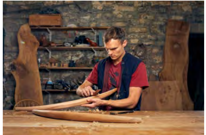
Finishing steam-bent Beech with Kanna
