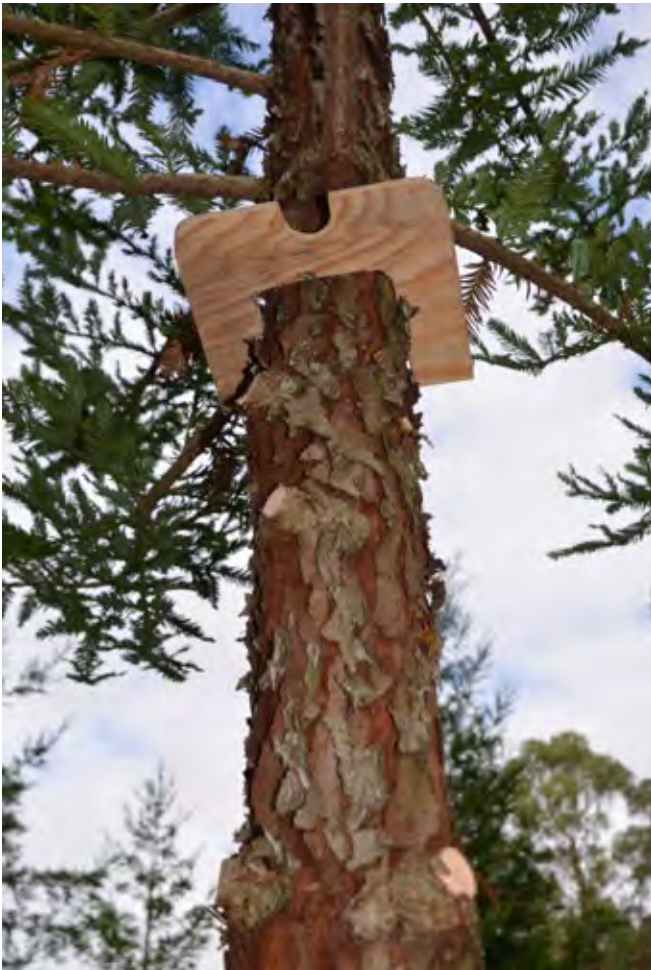
Rowan's pruning gauge, 8cm for stem pruning and 2.5cm for branch pruning
