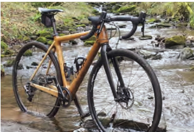
Ash used by Twmpa Cycles for a gravel bike frame
