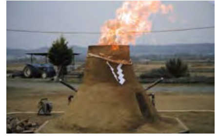
Tatara furnace used to make Tamahagane (steel)
