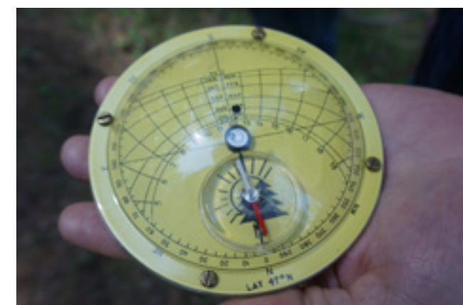
A solar compass used by foresters to achieve optimum exposure to direct daylight when designing canopy gaps created by group felling
