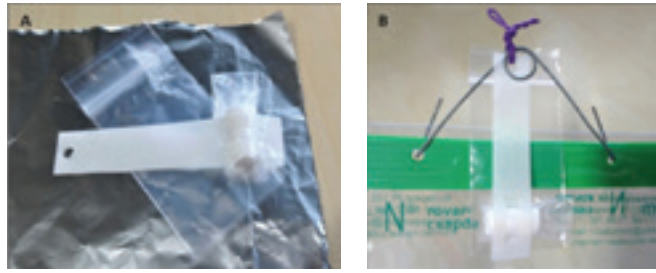
Figure 3 A: Dental roll / PE bag dispenser and small ziplock bag. B: Volatile lure attached to the hanging ring of a clear funnel trap.
