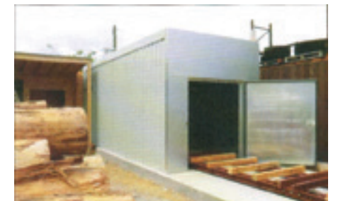
Small timber drying kiln with the capacity for 7 cubic metres of sawn timber
