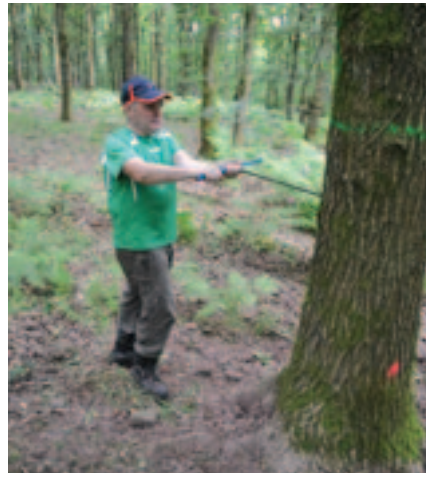
Core sampling for dendrochronological analysis at Chestnuts Wood. Pictured is Swansea University PhD students Neil Matthews and Josie Duffy
