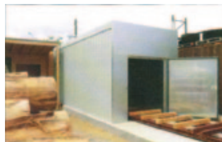
Small timber drying kiln with the capacity for 7 cubic metres of sawn timber
