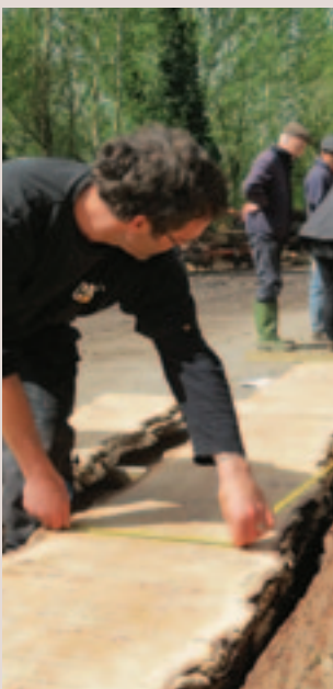
Measuring sawn timber
